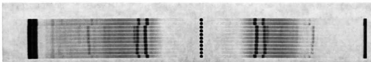
Fig. 2. Multiple-exposure powder patterns of adamantane under hydrostatic pressures around p_T ( p_T = 4800 \text{ kg cm}^{-2} ). Pressures ( \text{kg cm}^{-2} ): (from bottom) 1, 4500, 4600, 4700, 4800, 4900, 5000, 5100, 5200, 1 and 298 (released from 5200 \text{ kg cm}^{-2} ). Exposure time is 160 min for each exposed zone.
